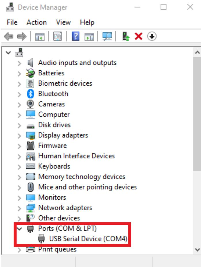
If you have multiple "USB Serial Device" entries, you may unplug the eGauge PRM3, and plug it back in to see which COM port appears when it is connected.
