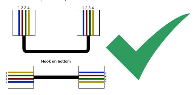
"Reverse" RJ-11 cable. This must NOT be used for the eGauge Sensor Hub.
