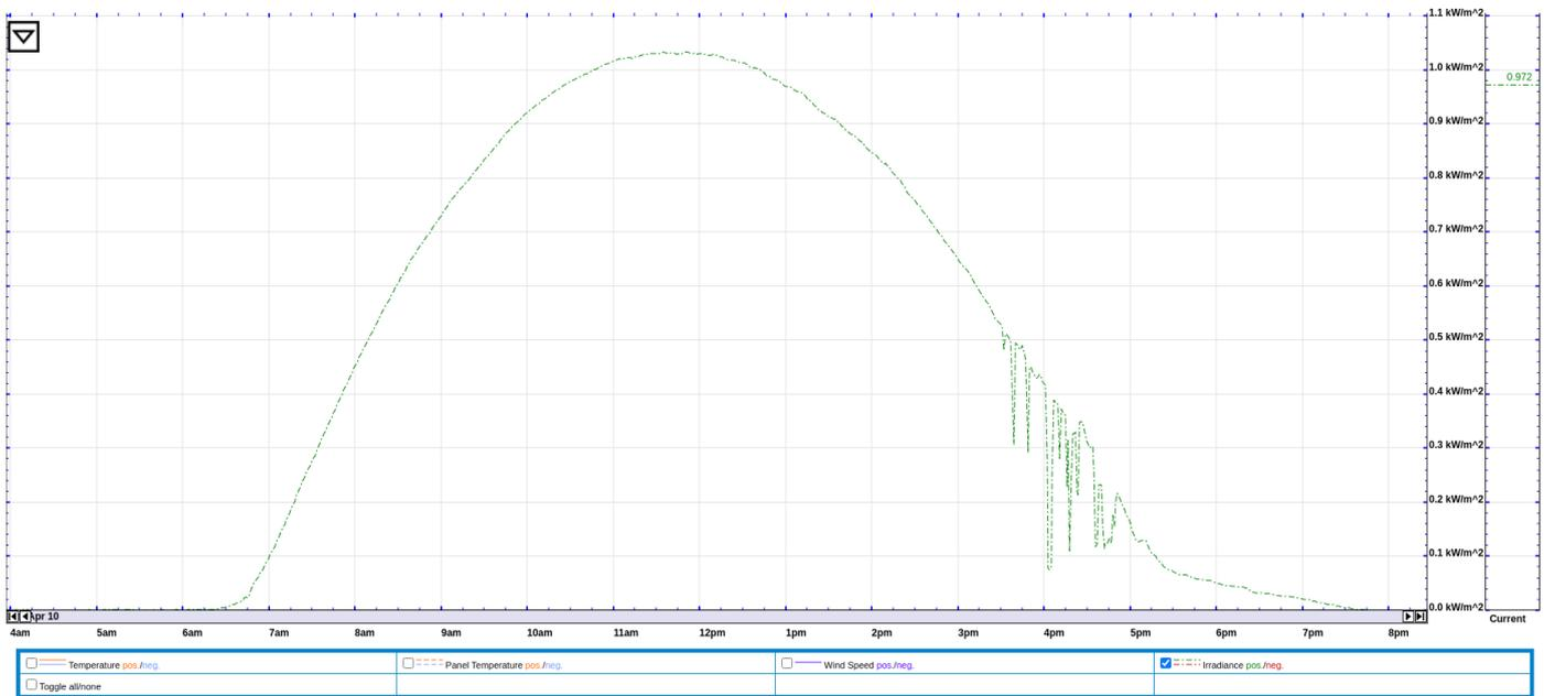
Data from the IMT sensor can also be used in formula registers to calculate the estimated solar production at a site. The formula for this calculation requires real time irradiance and temperature data (obtained from the IMT sensor), the array's rating in watts, and the panel temperature coefficient (usually a small negative number). The following example shows this formula based on a 10kW array and a temperature coefficient of  $-.12\%$ .
