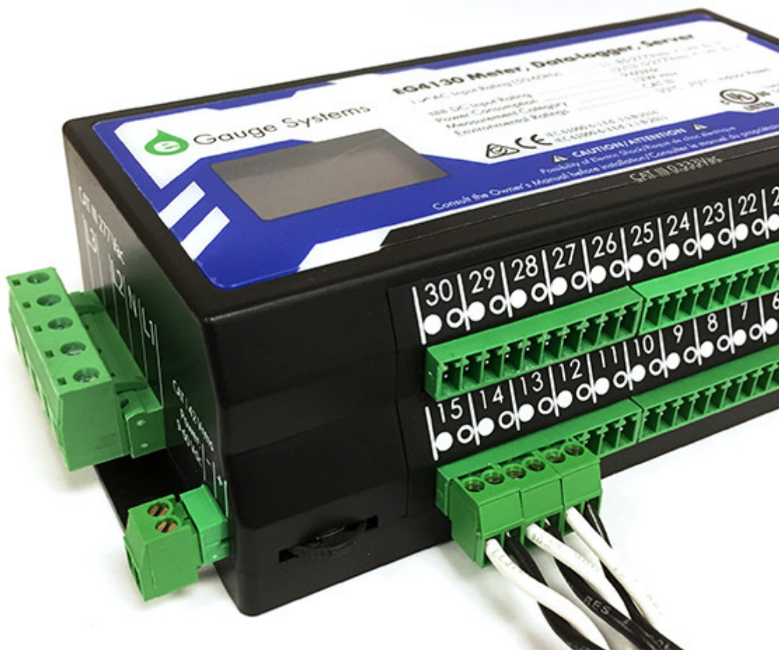
CTs connected to eGauge meter.
