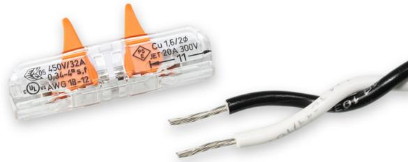
Lift the lever to insert the CT lead and lower the lever to secure the connection. You should use 1 inline connector per lead wire, using 2 inline connectors and 1 carrier to extend a single CT lead.
