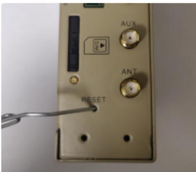
2. Use a push-pin or paperclip to hold down the "Reset" button on the side of the modem until the "STATUS" LED starts flashing and the "ERROR" LED remains solid, then release the button.
