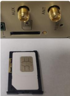
The cellular antennas must be located on the outside of any enclosure. Even plastic enclosures can degrade or block a cellular signal.
