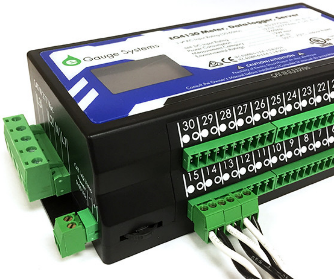
CTs connected to eGauge meter.
