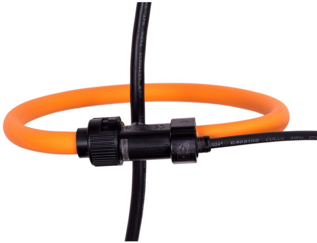
Conductor through center of rope CT (ideal placement)
