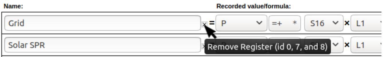
Grid is recording net power (=), positive-only (+) and apparent power (\*). They are recording in ID #0, #7, and #8 respectively.
